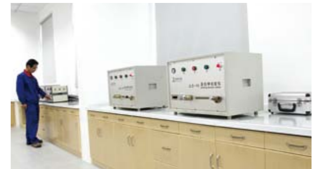
Jerking tension tester 急拉伸测试仪
