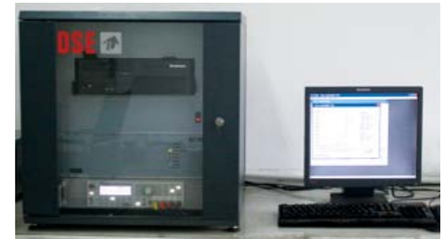
Dielectric loss tester 介质损耗测试仪
