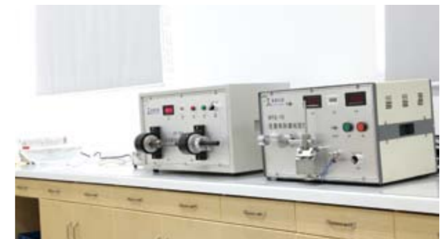
Scrape resistance tester 往复耐刮磨测试仪
