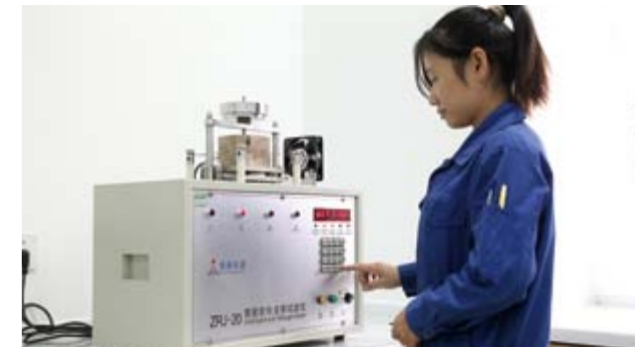
Intelligent cut-through tester 智能软化击穿测试仪
